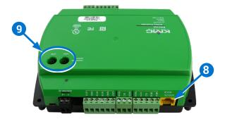
2. Wire any additional sensors to the **green (input)** terminal block 10. See Sample (BAC-9311) Wiring on page 7.
