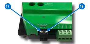
**NOTE:** Connect only one controller to each transformer with 12–24 AWG copper wire.
