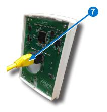
Plug an Ethernet patch cable 7 connected to an STE-9000 Series or STE-6010/6014/6017 sensor into the (yellow) ROOM SENSOR port 8 of the controller.
