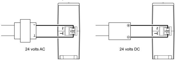
**For 24 volt AC power** Connect a 24 volt transformer to the black power terminal block on the end of the router.
